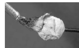
Thin slip with water and apply with a brush to the bead core. Dry and fire.
